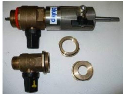
The penetration of BLUTOP tool into the pipe will be done by manual push of the operator.
