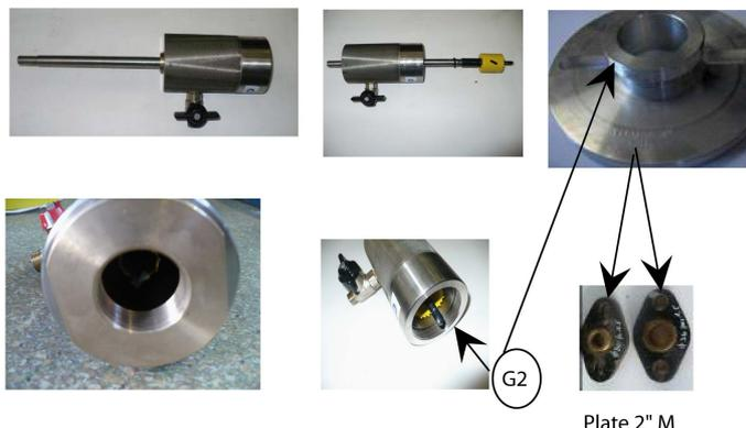
The plate 2'M with flange is screwed on G2 and allow the installation of PM and GM flange adapters.
